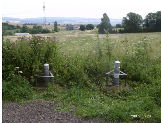
Groundwater measuring points within different depths at measuring point Bakede
