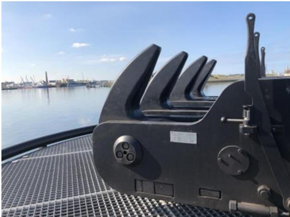
Abbildung 7-2: Example Quick release hook (Source: Straatman)
