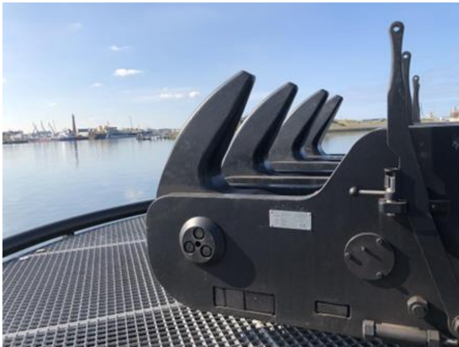
Abbildung 7-2: Example Quick release hook (Source: Straatman)
