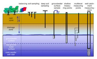
Instruments for efficiency control in soil and groundwater
