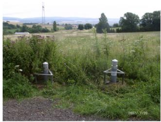
Groundwater measuring points within different depths at measuring point Bakede
